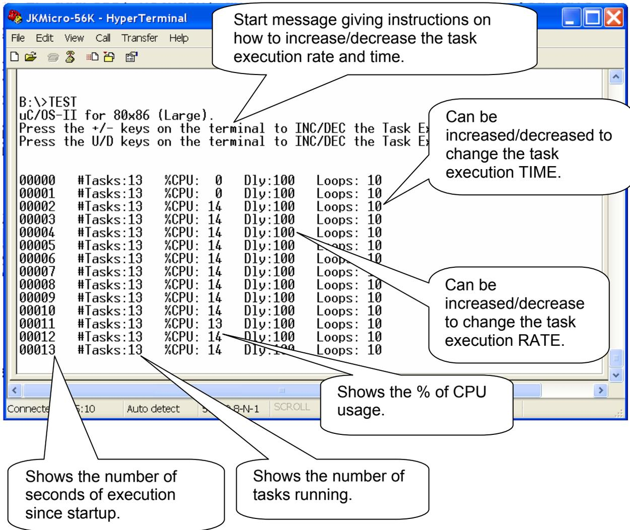
Figure 3, Running TEST.EXE on the μFlashTCP.
