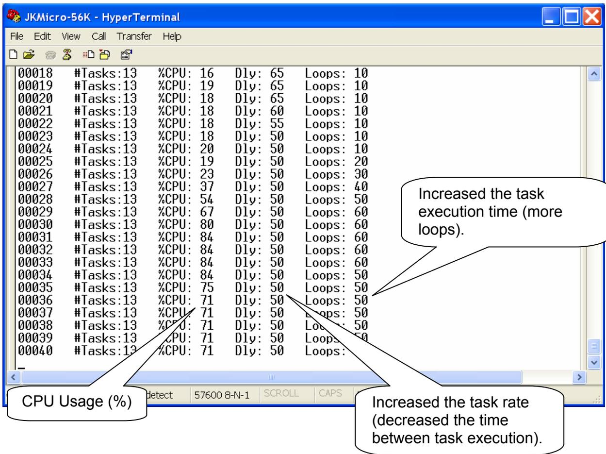
Figure 4, Increasing the task rate and execution time.
