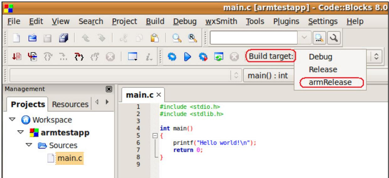
Change the Built target type to our armRelease target we just set up.
