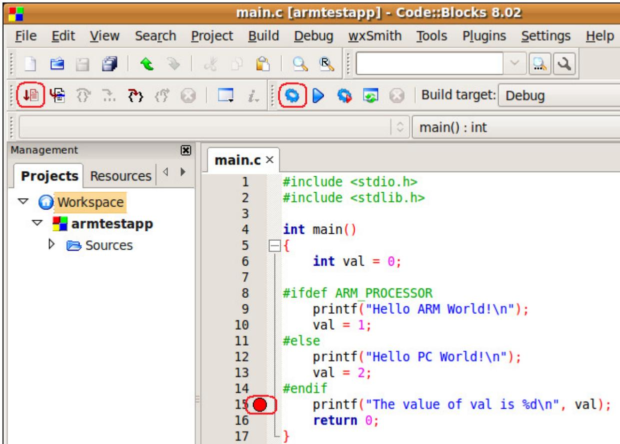
This picture shows setting a breakpoint, building the application, and then running it in debug.
