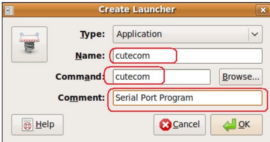
The Command is the most important here. Type cutecom. Give it a name and a comment and press OK. Then close the Add to Panel window.
