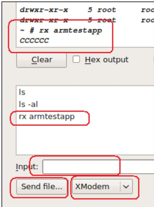
The first thing we do is type "rx armtestapp" or whatever the name of the program we want to receive on the ARM processor. We then press ENTER. This sends the receive X-Modem command to the ARM processor. The ARM processor starts querying for the file to be received. You will see at the top of the screen shot that the ARM received our command and the CCCC lets us know it is retrying to receive the file. Next we change the file type to XModem and click the Send file... button.
