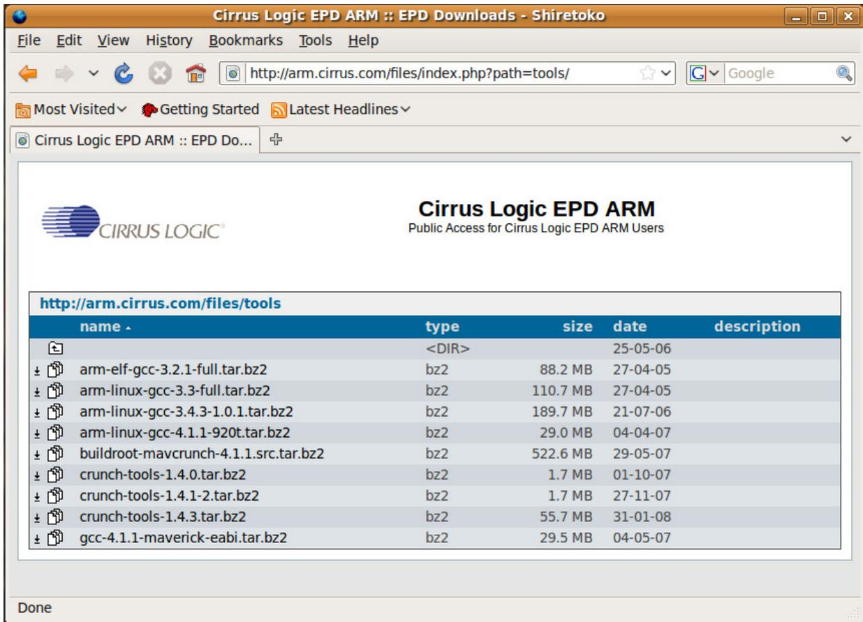
For the **OmniFlash**, download the "**arm-linux-gcc-3.3-full.tar.bz2**" file. For the **OmniEP**, download the file "**arm-linux-gcc-4.1.1-920t.tar.bz2**". I haven't played around too much with compiling for the OmniFlash with the 3.43 or 4.1.1 compiler yet. It may work.
