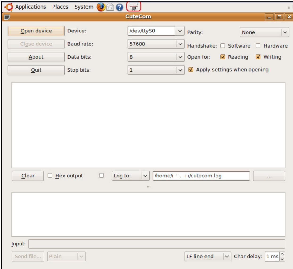
**Note: Make sure you close PuTTY before you do this as only one program can be connected to the serial port at a time.**
