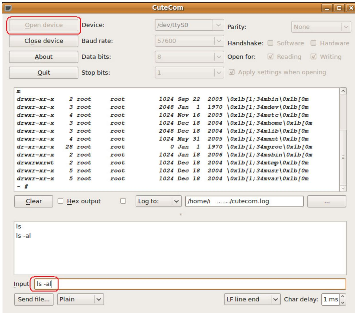
On the input line, we can type commands. Pressing Enter will send them. Once we send a command, we can double-click it from the lower window list.
