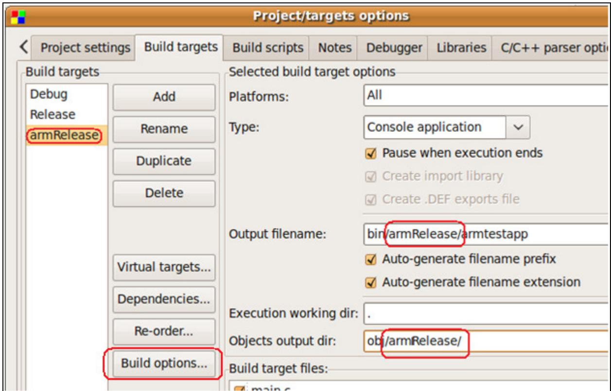
Make sure you have the armRelease target specified from the Build targets. Now add this name to the "Output filename" and "Objects output dir" or you will overwrite your regular release objects.
