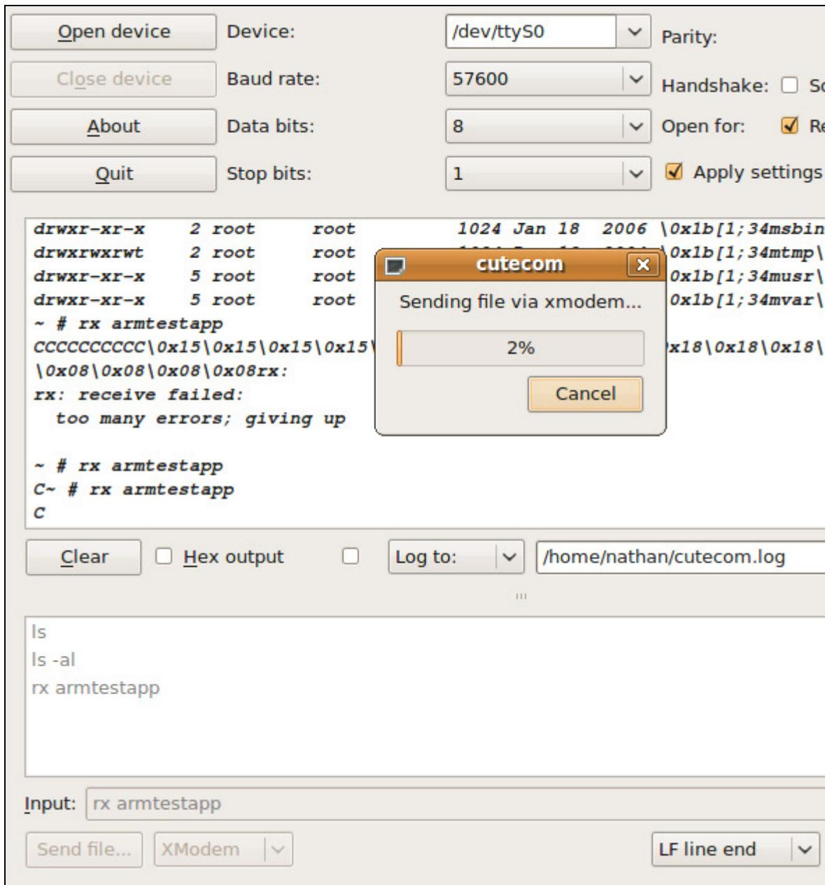
Here, I double-clicked on the "rx armtestapp" text which sent it to the ARM processor. Then I clicked the "Send file..." button and selected my test application. You can see that the file is being transferred to the ARM processor.
